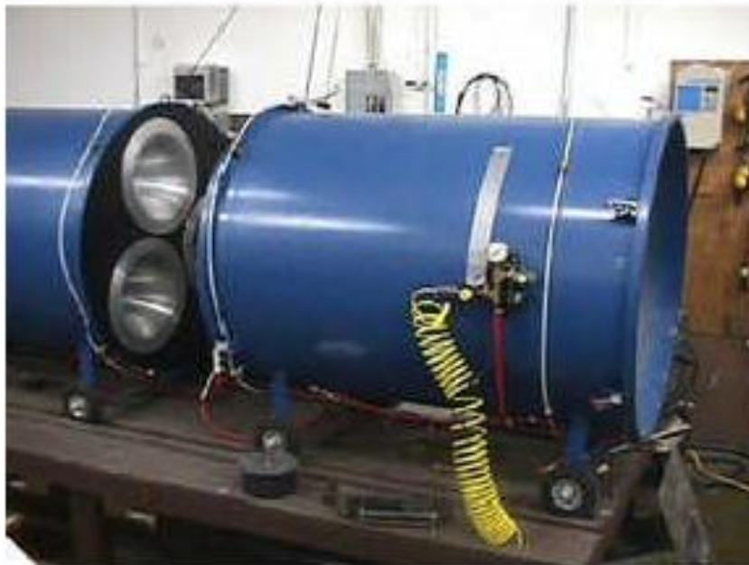
Figure C1, AMCA210-99 2000CFM Tunnel (Airflow Measurement Systems)
